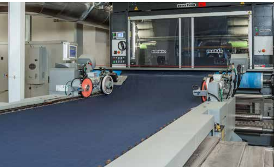
The Orthomax at Lanificio Ermenegildo Zegna and fili SPA removes web distortions before the stenter
