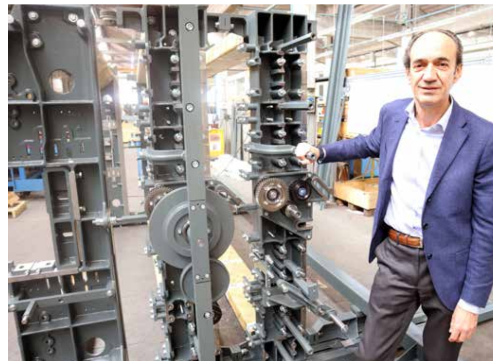
Giacomo Meucci with new cast iron frame used to assemble new cards – achieving stable setting between cylinders and drums.
