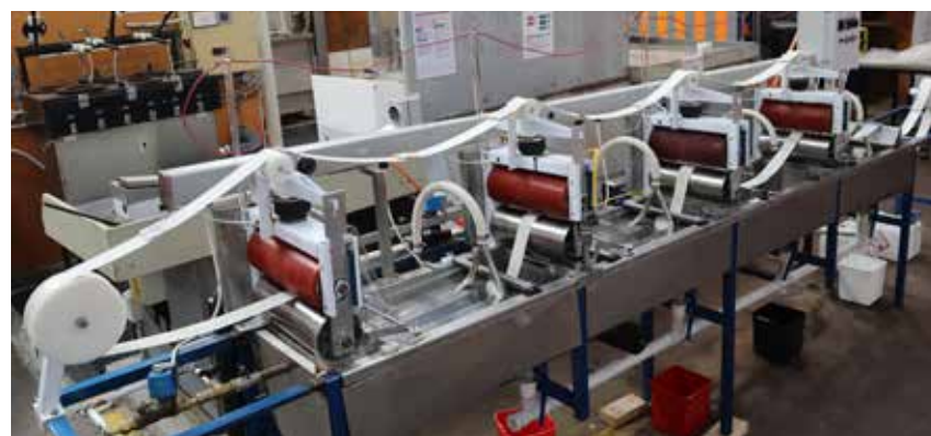
Mini wool scouring line specially built for SGS to test wool performance through the scouring process
