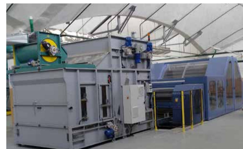
Schlumberger worsted card with new volumetric hopper-feeder developed with Tecnomeccanica Biellese
