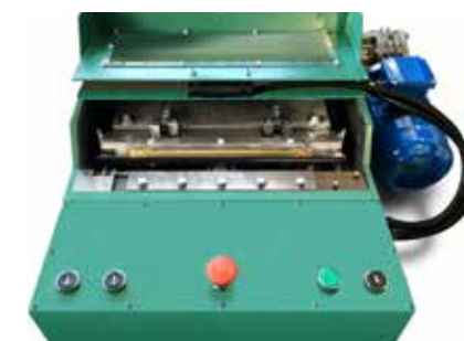
The insert grip can be adapted to any length of comb for chain gills
